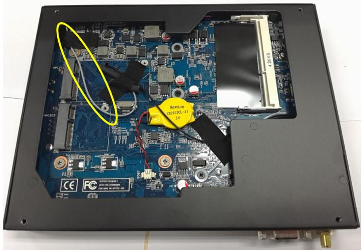
Unscrew (anti-clockwise) the screws from Top panel of the PC and remove the Top panel (be careful the inner antenna which for BT).
