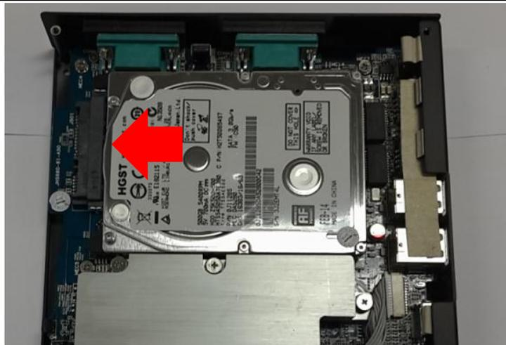
Turn over the whole PC, and fix the HDD with 3 HDD screws as the picture shown.
