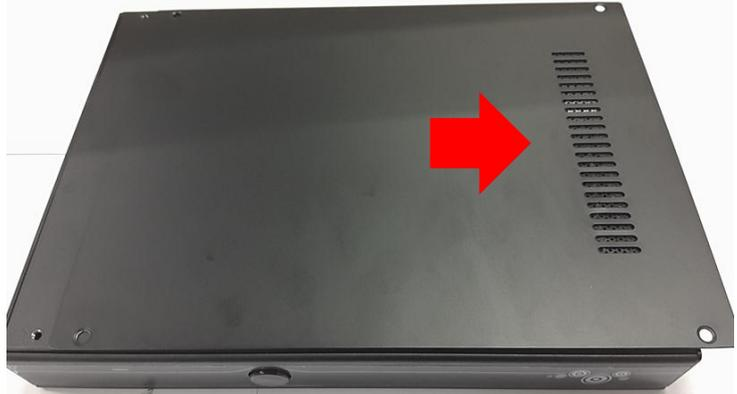
If you need to install HDD, you need to release the inner antenna which connected to the top panel, and then to remove the top panel.
